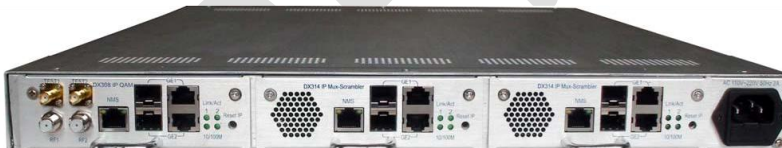
One OX308 8 in 1 IP-Mux QAM module and two OX314 12 channel IP input and 4 TS output IP-Mux Scrambler Modules. (8 channel QAM carrier and 8 Mux-scrambling IP output in all)
