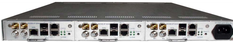
Three OX308 8 in 1 IP Mux-QAM Modules (24 QAM Carrier in all)
